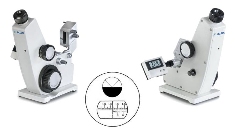
This model is a simple Abbe refractometer with thermometer and is extremely reliable. You can evaluate liquid samples, solid samples as well as paste samples. Key features of this refractometer are its sturdiness and its ease of use.
